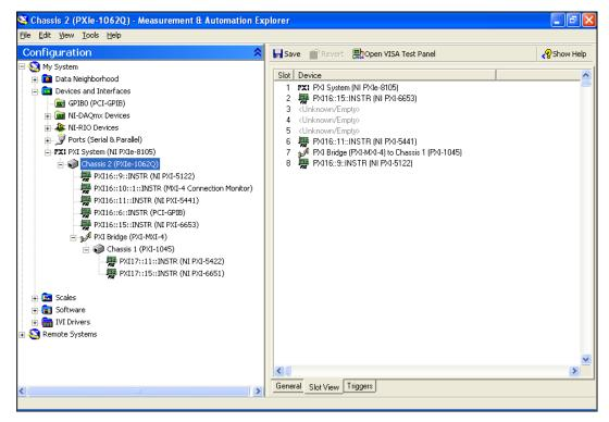
Figure 2-4. Multichassis Configuration in MAX
